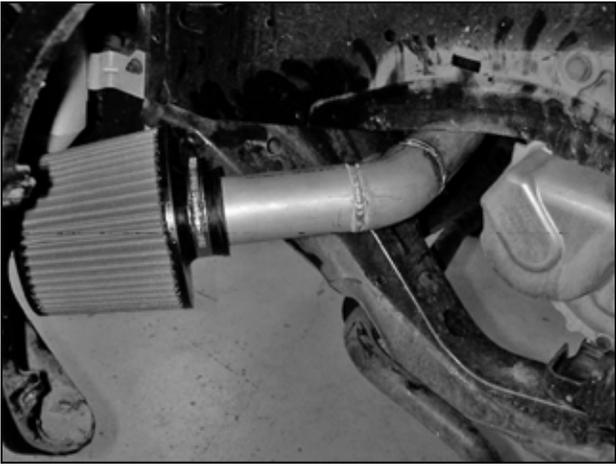
e. Install the air filter onto the intake pipe and secure with the provided hose clamp. Adjust the air filter for best fitment and ensure sufficient clearance.
