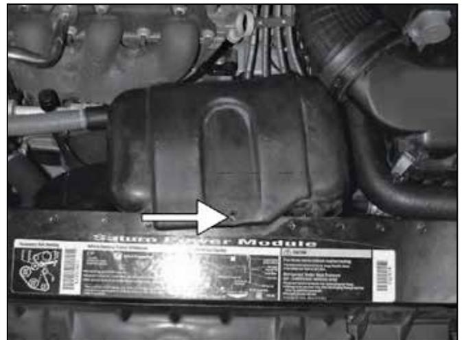
b. Remove the plastic clip from the resonator. Remove the resonator from the vehicle.
