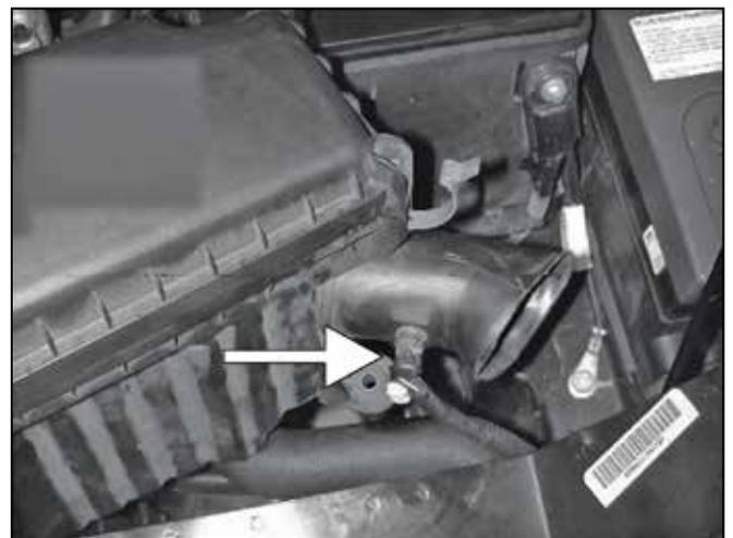
d. Unplug the IAT from the factory air box. Remove the air box from the vehicle.
