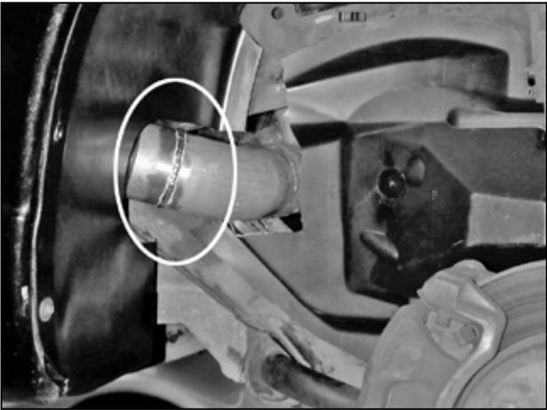
g. Attach the outer fender liner to determine where it will make contact with the intake pipe. The outer fender liner will need to be trimmed to clear the intake pipe. Once the liner is trimmed and provides adequate clearance, install the liner and the hardware needed to secure it in place.
