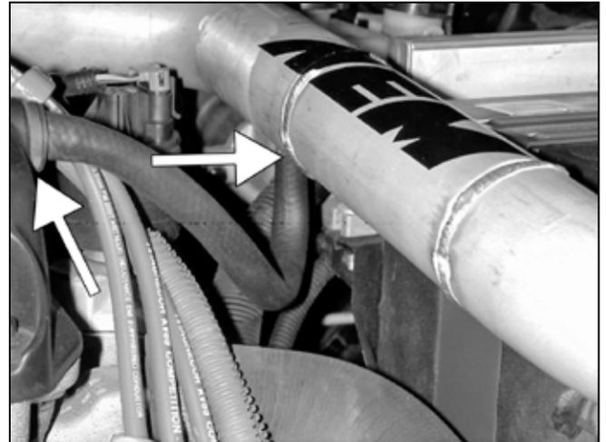
c. Attach the crankcase breather hose to the valve cover and the intake pipe.
